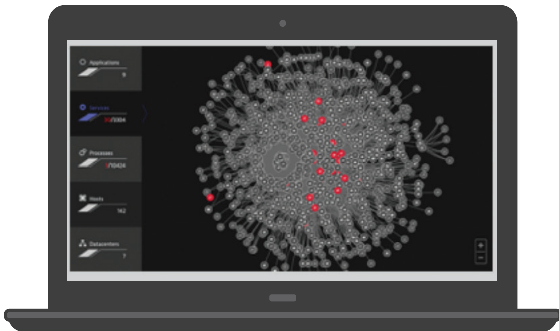
Figure 1. Dynatrace Smartscape view of a complex microservices environment. Multiple failures are in red, but the display also confirms that system redundancies prevented any end-user impact
